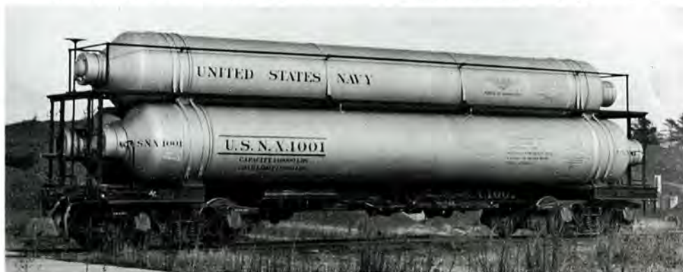
USNX 1001, the only U.S. Navy three-tube car at Lakehurst, New Jersey, November 2, 1926. Two others were built by Bethlehem for the Army Air Service. — Navy Bureau of Aeronautics
