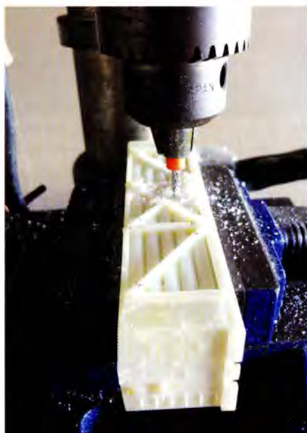
Fig. 4 Using my drill press as a mill to remove the cast-in X-bracing a little at a time.
