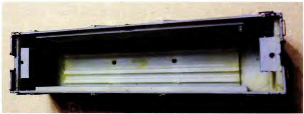
Fig. 11 Blocks at the ends of the shell have been drilled to hold the coupler boxes and floor to the car body. These are set so the new floor will be level with the shelves cast inside of the model where the original floor rested. The end sills have been notched for the new coupler height.
