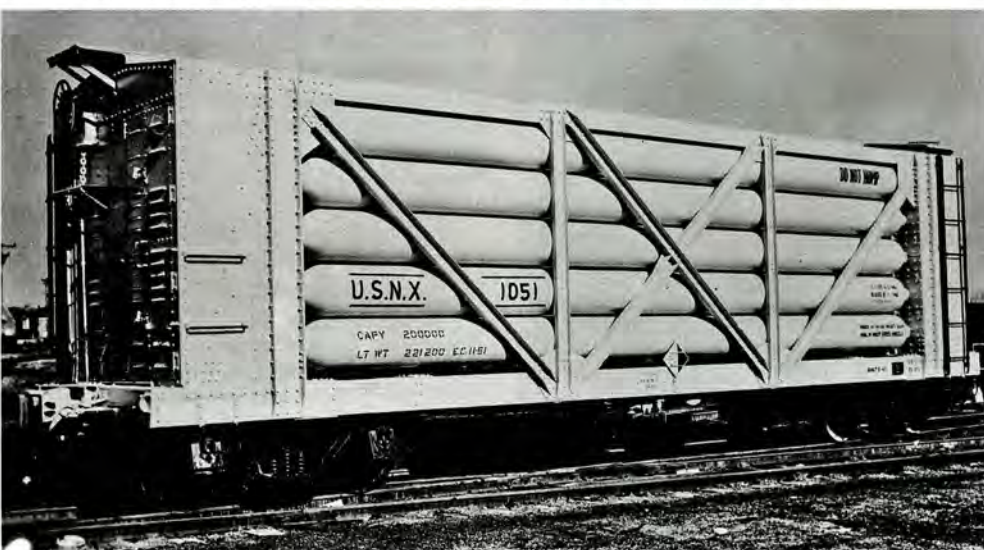
One of 65 World War II-era 30-tube cars built by GATC in 1942-1943. With only minor modifications, this was to become the pattern for all future helium tank cars. — GATC photo, U.S. Bureau of Mines, National Archives and Records Administration, Ft. Worth
