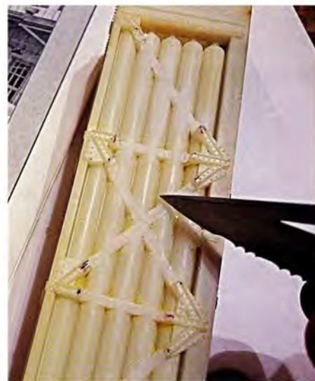
Fig. 6 A curved blade was used to remove the last of the castings to flush with the tubes.
