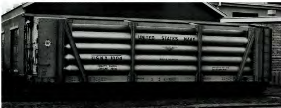
USNX 1004, one of five 28-tube cars built by GATC in 1930, at the Amarillo helium plant circa 1934. — U.S. Bureau of Mines, National Archives and Records Administration, Ft. Worth
