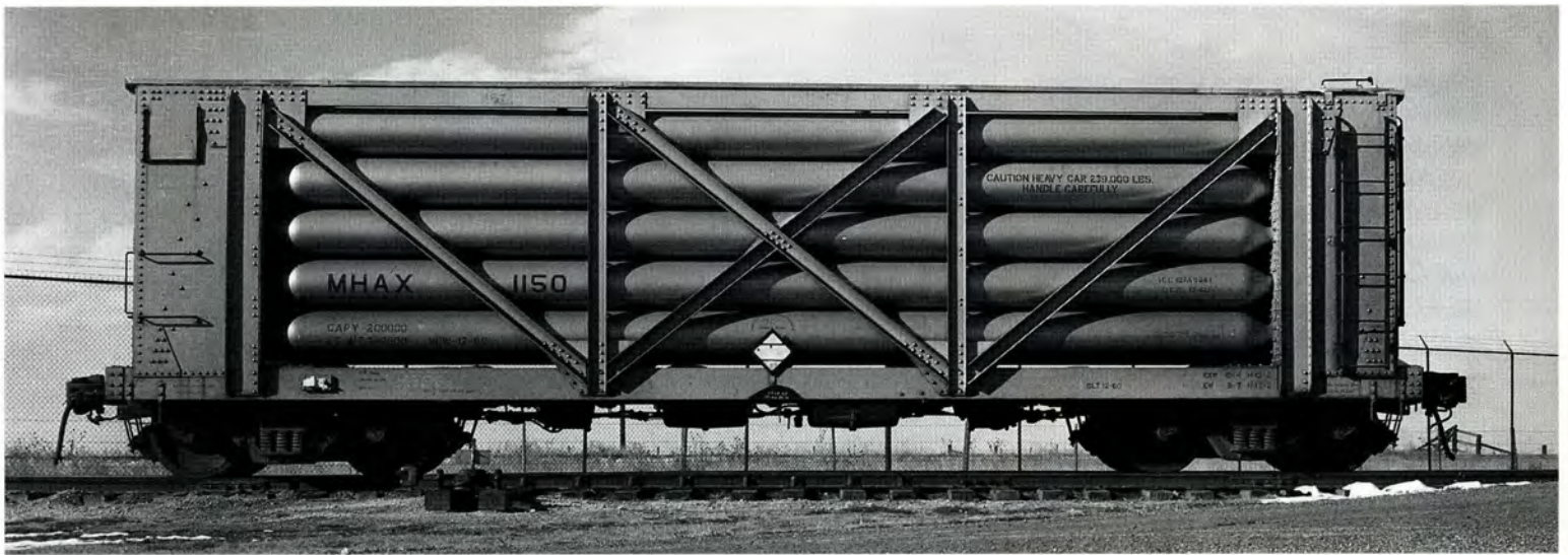
MHAX 1150, was built by ACF in 1960 and is seen here at Exell on November 19, 1962. The car was delivered with the heavy-duty trucks fitted with roller bearings and a metal roof walk. Notice how low it sits on the trucks. —U.S. Bureau of Mines, National Archives and Records Administration, Ft. Worth
