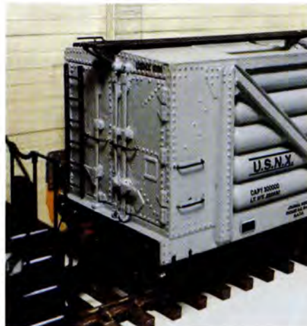
Figs. 9 & 10 The AHM A End casting, and as modified with strip brass shapes and new ladder.
