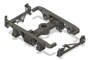
Install the wheel sets into the trucks by gently spreading the sides of the truck. Then attach the brake ends to the truck. They might have a tight fit that will require a little bit of careful force. I recommend only gluing one side of the brake end to allow spreading the truck to paint or replace the wheels later. Fill in attachment holes if the brake ends are not used.
