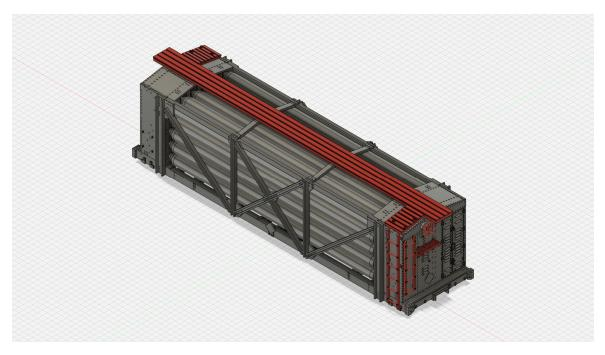
Next, attach the roof walk and all 4 ladders (see notes). Attach the brake stand and brake wheel.
