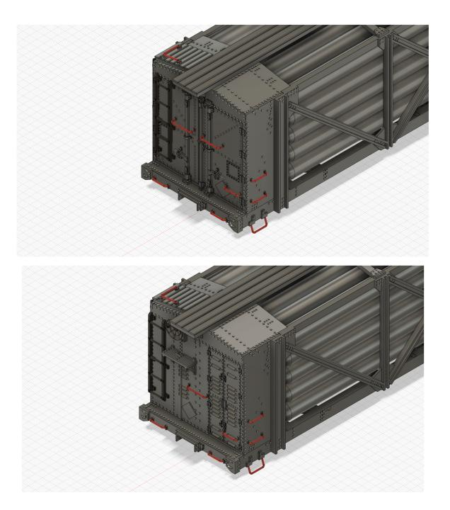
Next, attach grab irons, if not already installed prior to painting. These can be trimmed, as needed. A #80 or #79 drill might be needed to clean out the holes.
