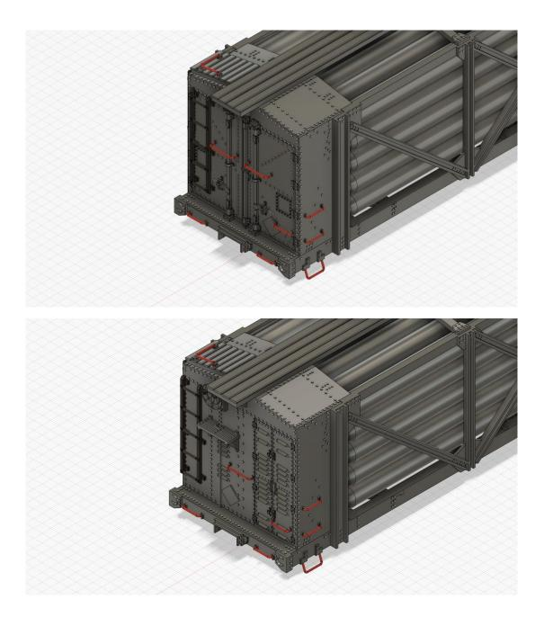
Next, attach grab irons, if not already installed prior to painting. These can be trimmed, as needed. A #80 or #79 drill might be needed to clean out the holes.
