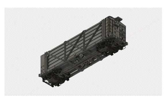
Install the couplers onto the frame with the black screws and Kadee coupler covers.
