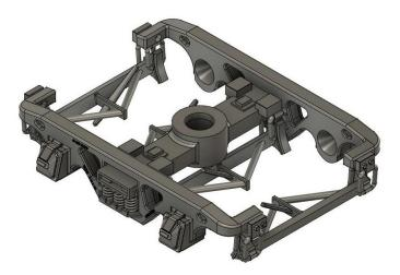
Decide on which set of trucks to use. The older solid "friction" bearing version is shown. Roller bearing trucks were required for interchange service by 1991. Install the wheel sets into the trucks by gently spreading the sides of the truck. Then attach the brake ends to the truck, if needed. They might have a tight fit that will require a little bit of careful force. I recommend only gluing one side of the brake end to allow spreading the truck to paint or replace the wheels later.
